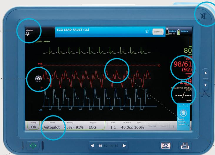
Illuminating switch indicates pump is alarming and the priority level
