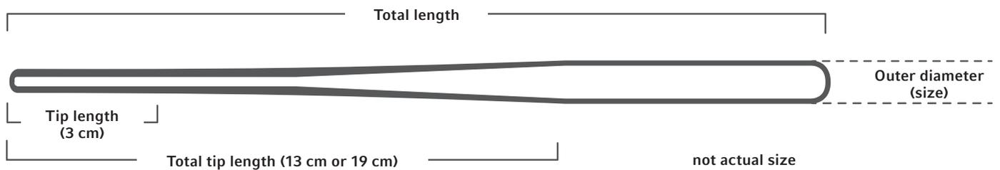
**FLEXIBLE NITINOL GUIDEWIRES WITH STRAIGHT STANDARD TIP (13 CM)**
